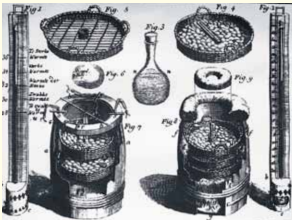
Barrel incubator, ca. 1750, heated with dry manure. An invention from Réaumur.
