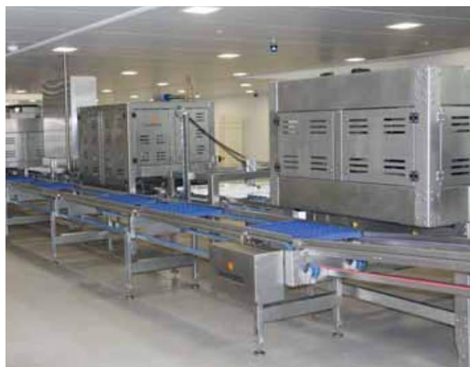
Candling line of Innovatec, including the CleanChick system. PHOTO: TOM SCHOTMAN, AGRIO
